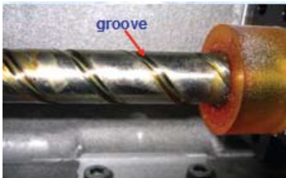
Figure 6 : Zone of Conflict on Lead Screw Groove
