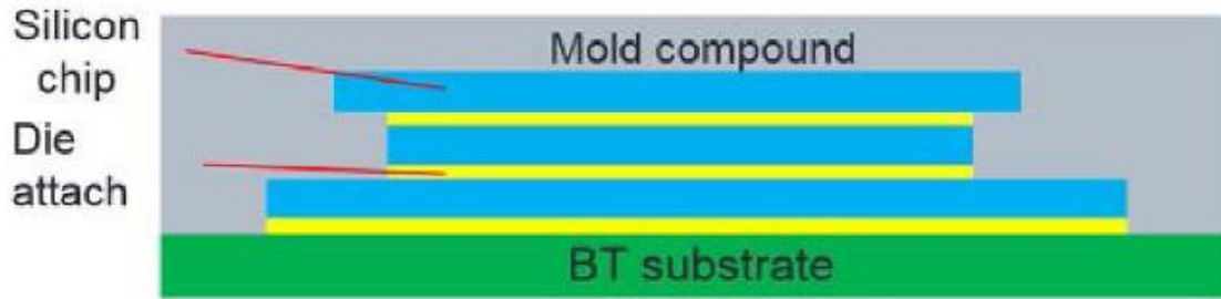
Figure 2.3 Schematic of the stacked die package. Source: Wang (2016).
