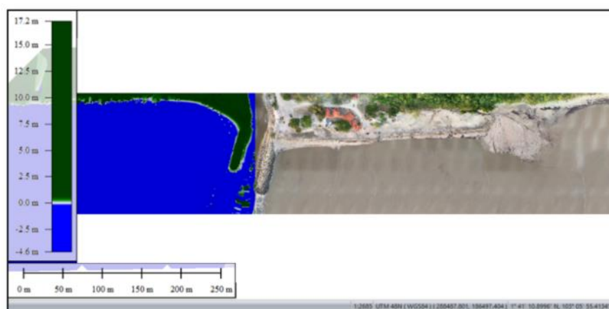
Figure 7. NDVI Layer in Global Mapper to determine shoreline.
