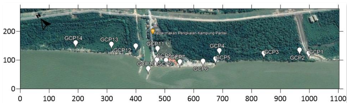
Figure 4. The location of GCPs along the shore of Pantai Punggur.
