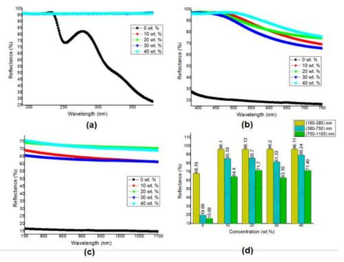
**Figure 5.** UV-VIS reflectance spectra of PVA/molasses composite at different concentrations of molasses (0, 10, 20, 30 and 40 wt.%)
