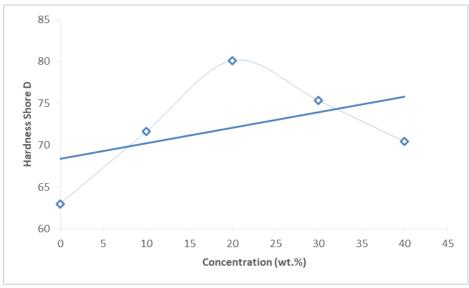
**Figure 12.** Hardness shore D average of PVA/molasses composite at different concentrations of molasses (0, 10, 20, 30 and 40 wt. %)
