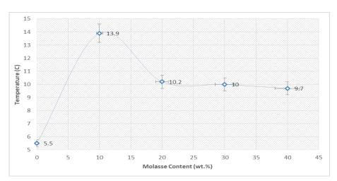
**Figure 11.** Difference maximum temperatures curve between before and after demonstration of sun light for 1 minute of PVA/molasses composite by IR camera at different concentrations of molasses (0, 10, 20, 30 and 40 wt.%)
