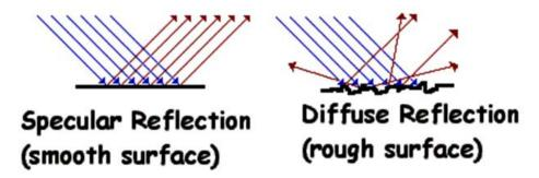
Figure 9. Schematic shape of smooth and rough surface and it is affecting on magnetic waves reflection
