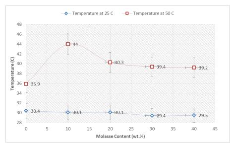
**Figure 10.** Maximum temperatures curve of PVA/molasses composite by IR camera at different concentrations of molasses before and after demonstration of sun light for 1 minute (0, 10, 20, 30 and 40 wt. %)
