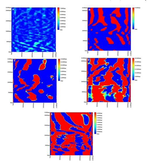
**Figure 6.** AFM 2D topography images of PVA/molasses composite at different concentrations of molasses (0, 10, 20, 30 and 40 wt.%)
