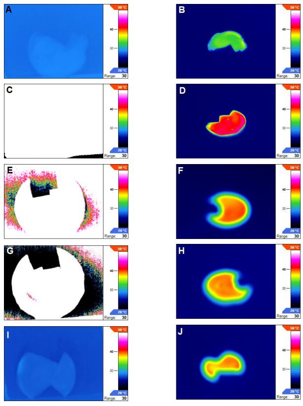
**Figure 8.** IR images of PVA/molasses composite by IR camera at different concentrations of molasses (A and B=0, C and D=10, E and F=20, G and H=30, as well as I and J=40 wt.%), before and after demonstration of sun light for 1 minute, respectively
