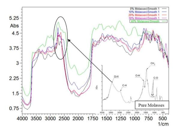
**Figure 2.** FTIR absorption spectra of PVA/molasses composite at different concentrations of molasses (0, 10, 20, 30 and 40 wt.%)
