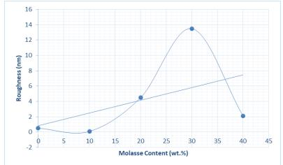
**Figure 7.** Roughness average curve of PVA/molasses composite surface by AFM at different concentrations of molasses (0, 10, 20, 30 and 40 wt.%)
