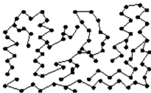
Figure 2.1: Illustrative structure representative of LDPE (Durmus et al, 2007).
