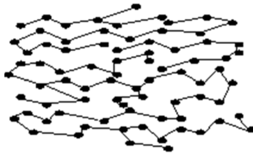
Figure 2.3: Illustrative the structure representative of LLDPE (Durmus et al, 2007).
