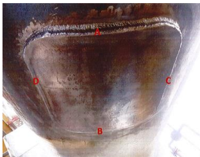
Figure 8. Location for Hardness Test after Fillet Weld.
