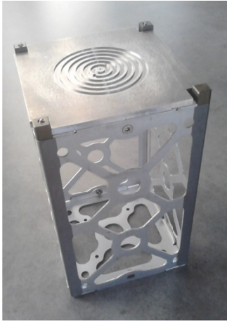
FIGURE 5: The Bull's Eye antenna on a CubeSat chassis [57].
