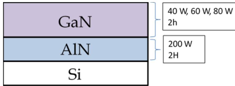
Figure 1. Schematic of GaN/AlN films grown on Si (100) substrate.
