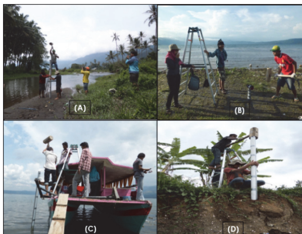
Figure 2: PVC core sampling process on various lands: (A) Point bar, (B) Lake beach, (C) Lake dash, and (D) River terrace
