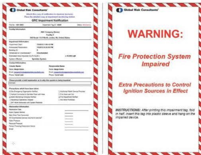
Figure 3: Sample of a fire protection impairment permit. On the left is the front with the impairment data and right is the back with the warning details.
