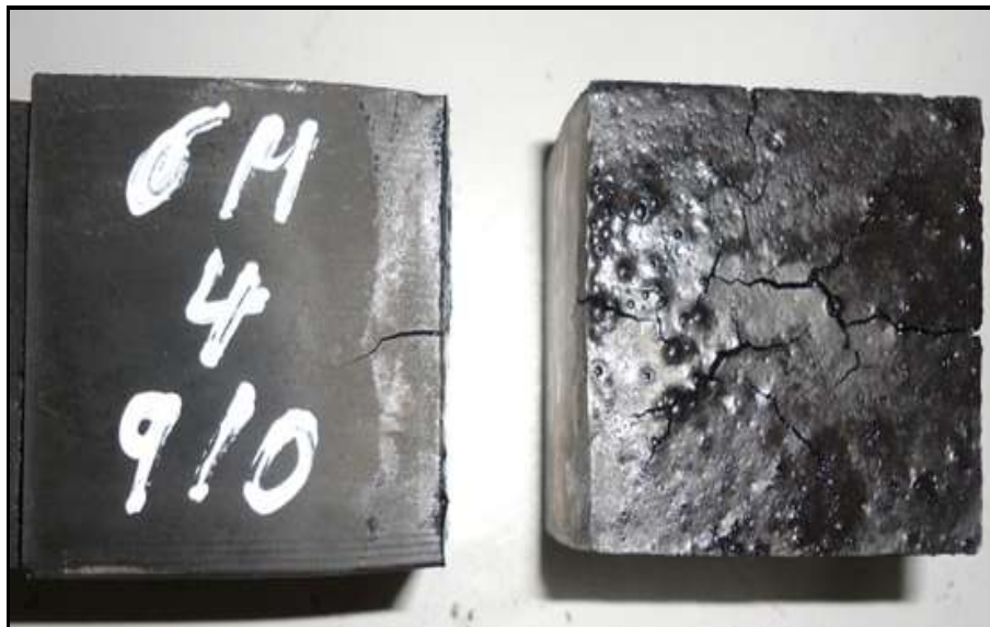
Fig. 3: Cracks on the top of specimens after 24 hours oven curing.
