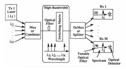
Figure 2.4: Diagram of a Simple WDM System
