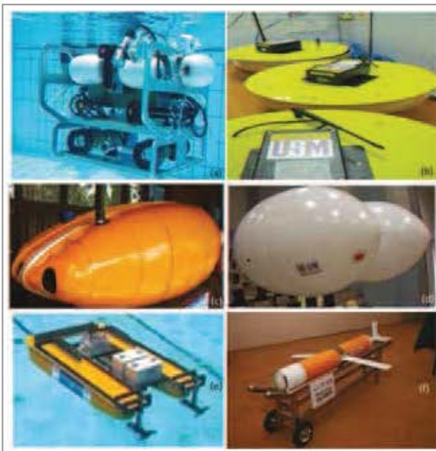
Figure 2: Underwater robotic platforms for ocean observation (a) Mini Remotely-Operated Vehicle (ROV), (b) Drosobots, (c) IHUV, (d) Blimp, (e) ASV, (f) Glider
