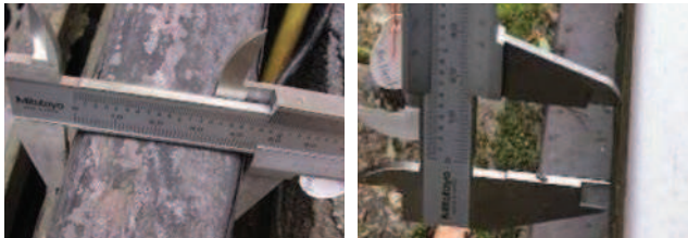
Figure 4: Rails width worn off by 5mm and rail head worn off by 1mm
