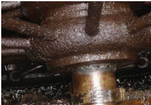
Figure 5: The over-welded bull wheel
