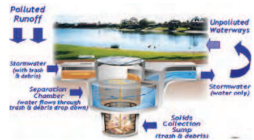
Figure 2: CDS unit in stormwater treatment operation
