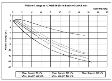
Figure 14: Volume change for specimen of particle size 0.6 mm
