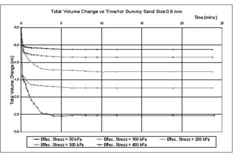
Figure 5: Total volume change during isotropic compression for grain size (0.6 mm)
