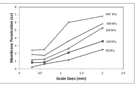
Figure 12: Comparison of membrane penetration relation to grain sizes (0.3, 0.6, 1.18 and 2.0 mm) under different effective confining stress (50 – 400 kPa)
