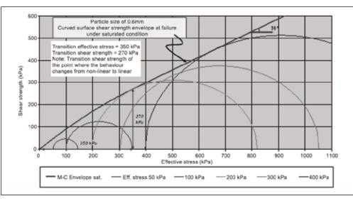
Figure 15: Curved surface shear strength envelope at saturation for particle size of 0.6 mm
