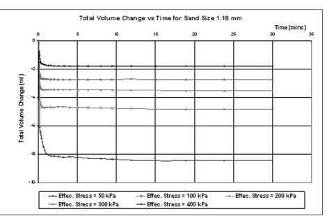
Figure 6: Total volume change during isotropic compression for grain size (1.18 mm)
