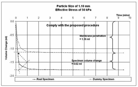
Figure 10: Graphs of isotropic consolidation on the dummy and real specimens of grain size 1.18 mm and effective stresses of 50 kPa
