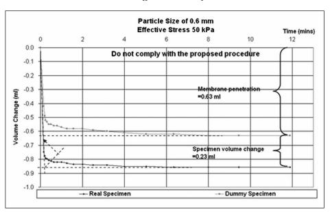
Figure 9: Graphs of isotropic consolidation on the dummy and real specimens of grain size 0.6 mm and effective stresses of 50 kPa
