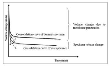
Figure 1: Schematic diagram to estimate membrane penetration isotropic consolidation curve
