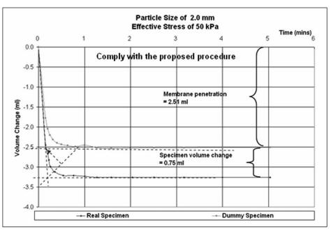
Figure 11: Graphs of isotropic consolidation on the dummy and real specimens of grain size 2.0 mm and effective stresses of 50 kPa
