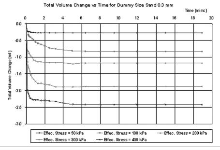
Figure 4: Total volume change during isotropic compression for grain sizes (0.3 mm)
