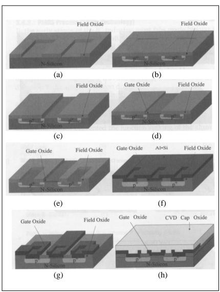
**Continue: Figure 3.2** Fabrication pocess step (a) after strip photoresist using acetone. (b) source/drain doping. (c) Form gate pattern using lithography process. (d) Grown gate oxide using dry oxidation. (e) Form contact pattern (f) deposit metal (aluminum) using PVD. (g) After aluminum etch. (h) Deposited passivation layer.
