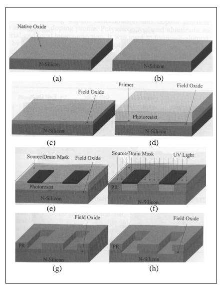
**Figure 3.1** Fabrication Process step (a) and (b) process wafer cleaning using BOE (Buffered Oxide Etch). (c) An oxidized Si wafer by wet oxidation. (d) Application of resist. (e) and (f) Resist exposure through the mask. (g) The wafer after the development. (h) The wafer after SiO<sub>2</sub> removal.
