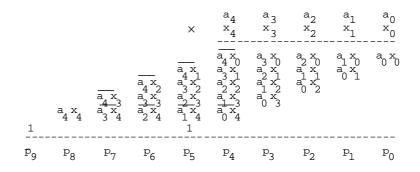
Figure 2.7 : Modified Baugh-Wooley Two's Complement Signed Multiplication
