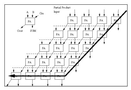
Figure 2.1 : 4-bits x 4-bits Array Multiplier [6]
