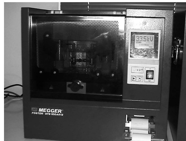
Figure 3: Dielectric breakdown voltage measurements equipment
