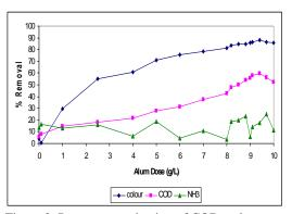
Figure 1: Percentage reduction of COD, colour and NH<sub>4</sub>-N vs PAC dose. Test performed at neutral pH.
