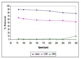
Figure 6: Percentage reduction of colour, COD and ammonia vs speed of rapid mixing. Tests performed with OpCD and pH of alum.
