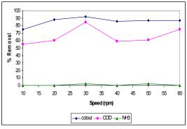
Figure 7: Percentage reduction of colour, COD and  $NH_3$  in different speed of slow mixing. Tests performed with OpCD, pH and rapid mixing parameter using PAC.
