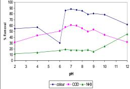
Figure 3: Percentage reduction of COD, colour and NH<sub>4</sub>-N vs pH. Tests performed with OpCD of PAC.
