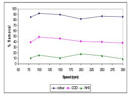
Figure 5: Percentage reduction of colour, COD and  $NH_3$  vs speed of rapid mixing. Tests performed with OpCD and pH of PAC.
