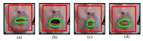
Figure 2.1: Sample result of mouth region (red rectangle) and lip shape detection (green ellipse) for the lack of the gesture (a) and for three gestures recognized: opening the mouth (b), making the mouth into an "o" shape (c) and sticking out the tongue (d) (Dalka and Czyzewski, 2009).
