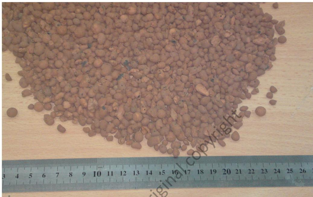
Figure 3.5: LWA used in the manufacturing of the LWAGC of this study.
