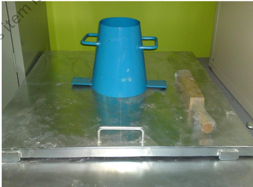
Figure 3.6: Slump test instrument used to test the fresh concrete slump.
