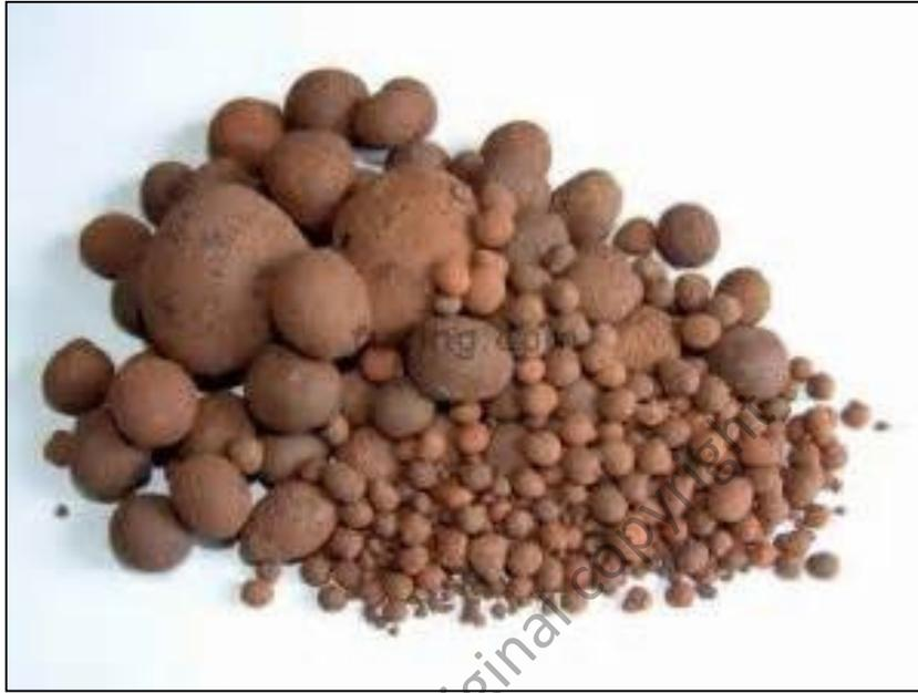
Figure 1.1: Expanded clay LWA.
