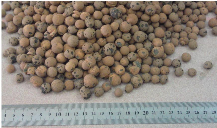
Figure 3.7: Batch 2 LWA of 8-16 mm.
