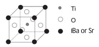
Figure 2.2: The ABO<sub>3</sub> perovskite structure of Ba<sub>x</sub>Sr<sub>1-x</sub>TiO<sub>3</sub> (Adikary, 2003)
