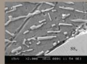
Figure 2b Magnified SEM micrograph of coarse acicular eutectic Si needle-shaped particle near to the double stainless steel wires.
