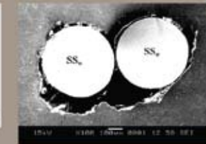
Figure 4 Debonding associated with large void around double stainless steel wires.
