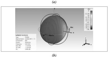
Figure 8: Simulated far-field patterns of E-shaped rectangular patch antenna: (a) polar form (b) 3-dimensional form
