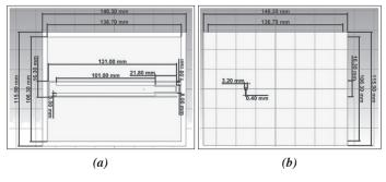
Figure 1: Configuration of rectangular patch antenna with modified U-slots: (a) top view (b) bottom view
