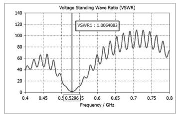
Figure 7: Simulated VSWR of E-shaped rectangular patch antenna
