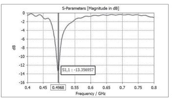
Figure 3: Simulated reflection coefficient of rectangular patch antenna with modified U-slots
