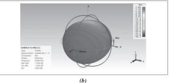
Figure 5: Simulated far-field patterns of rectangular patch antenna with modified U-slots: (a) polar form (b) 3-dimensional form
