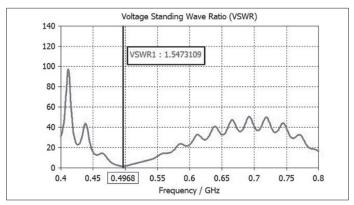
Figure 4: Simulated VSWR of rectangular patch antenna with modified U-slots
