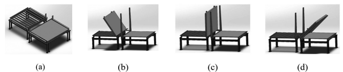
Figure 2-2: The flipping process was demonstrated: (a) resting table with two L-beams, (b) product on roller table being flipped up, (c) the flipped up product received by two L-beams of resting table, and (d) the product flipped and located on the resting table
