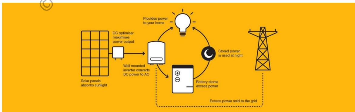
Figure 2.2: Solar Harvesting System using PV Modules ("How Solar works,")
