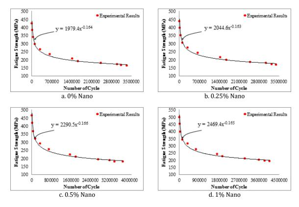
Figure 16. Curve fitting for experimental fatigue results with nanoparticle coating and laser treatment.
