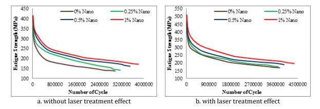
Figure 13. Fatigue characterizes material with and without laser treatment and nano effects.
