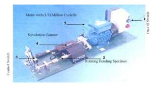
Figure 7. Bending rotating fatigue test machine.
