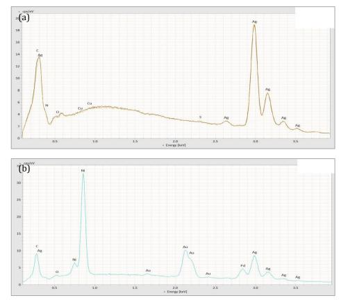
Figure 5. EDS spectra of; (a) standard Cu LF; (b) textured PPF-
