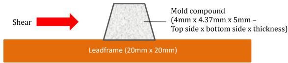
Figure 2. Schematic diagram of sample for mold shear strength test-
