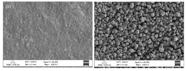
Figure 4. FESEM image of leadframe surface; (a) standard Cu LF; (b) textured PPF-
