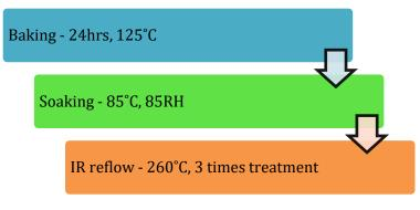
Figure 3. Process flow for pre-conditioning MSL level 1-
