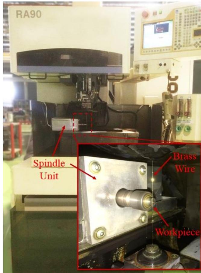
**Figure 1.** Non-submersible type of WEDM machine with precise spindle unit.
