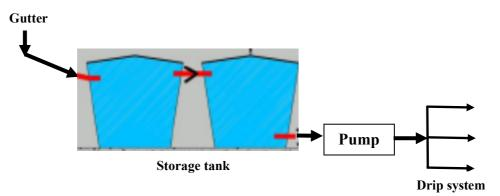
Figure 2. The developed irrigation system
