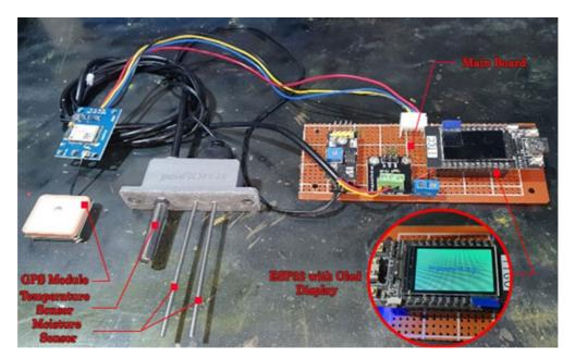
Figure 3. The Embedded Controller
