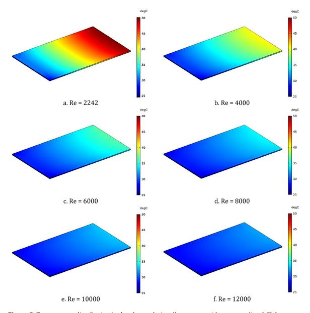
$\textbf{Figure 3.} \ \textbf{Temperature distribution in the photovoltaic cell structure with water cooling (°C) for a range of Reynolds numbers$
