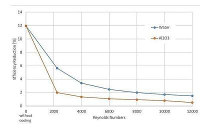
Figure 6. Photovoltaic electrical efficiency reduction as a function of Reynolds numbers
