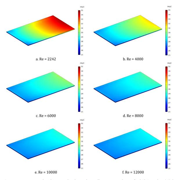
**Figure 4.** Temperature distribution in the photovoltaic cell structure with nanofluid Al<sub>2</sub>O<sub>3</sub> cooling (°C) for a range of Reynolds numbers
