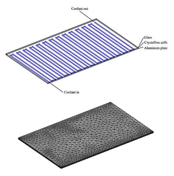
Figure 1. Computational domain and mesh of the photovoltaic cell panel
