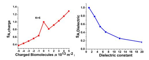
Fig. 5. Varying ambipolar sensitivity corresponding to (a) charged bio-molecules and (b) dielectric constant
