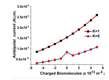
Fig. 4. Varying ambipolar current corresponding to charged biomolecules at k=1 and k=5
