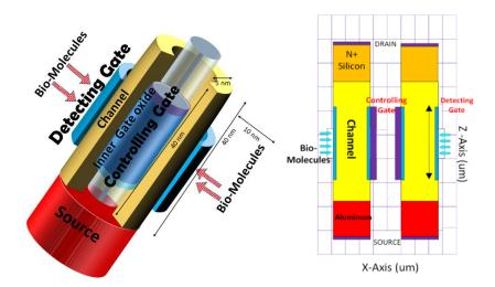
Fig 1. Silicon nanotube tunnel TFET biosensor illustration (a) 3D Inner and (b) vertical cross-sectional
