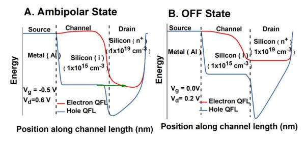
Fig 2. Quasi Fermi level for drain valance and channel conduction band at (a) ambipolar state and (b) OFF state
