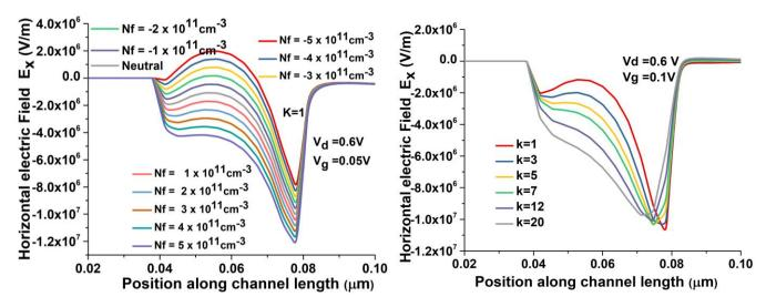
Fig 3. Electric field lines of SI\_NT\_TFET for various (a) dielectric constant (k) and (b) charged biomolecule ( $N_f$ )
