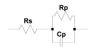
Figure 8. Equivalent circuit model
