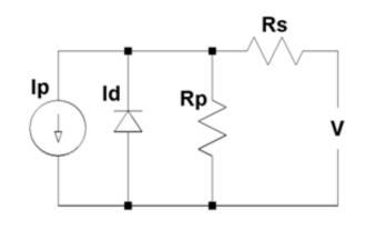
Figure 10. Diode model equivalent
