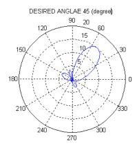
Fig.3.1 Radiation pattern of 4\*4 non-uniform planar array with 45° dx= $\lambda/2$ ;dy= $\lambda/4$
