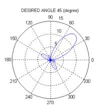
Fig.2.1 Radiation pattern of 4\*4 uniform planar array with  $45^{\circ}dx=dy=\lambda/2$ ,
