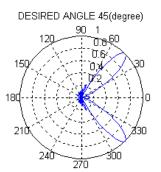
Fig.1.1 Radiation pattern of 16-element ULA with 45°
