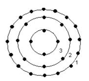
Fig.5 Modified Concentric Circular Array
