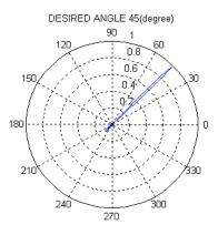
Fig.5.1.Radiation pattern of modified concentric circular array with 45°
