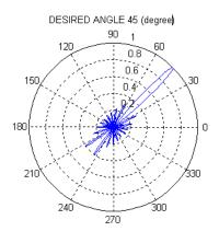
Fig.4.1.Radiation pattern of circular array with 45°
