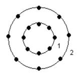
Fig.4. Concentric Circular Array-16 elements
