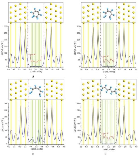
Figure 6.LDOS of "Au - (1,3-CHD→1,3,5-HT) - Au" nanodevice
