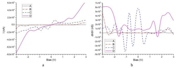
Figure 7.Current-voltage (a) and dI/dV characteristics (b) of nanodevices "Au − (1,3-CHD→ 1,3,5-HT) − Au"
