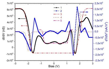
**Figure 8.**Phonon characteristics of a nanodevice "Au - 1,3,5-HT - Au" (D-configuration): 1 - differential conductivity of D-nanodevice, 2 - signals of the second derivative of the D-nanodevice, 3, 4 - dI/dV- and d<sup>2</sup>I/dV<sup>2</sup>-characteristics of the phonon system with a symmetric term (first mode), respectively, 5 - dI/dV-characteristic of a phonon system with a symmetric term (second mode)
