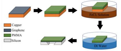
Figure 2. PMMA/Graphene film wet transferring process.
