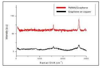
Figure 4. Raman shift of PMMA/Graphene membrane and CVD graphene on copper
