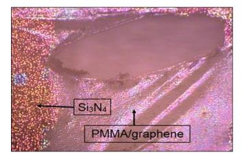
Figure 7. The tears of PMMA/Graphene membrane transferred by using 1.0M FeCl<sub>3</sub>.
