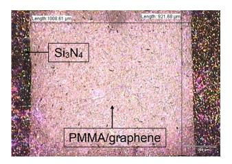
Figure 5. PMMA/Graphene membrane transferred by using 0.5 M FeCl3.
