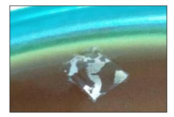
Figure 3. Etching process of CVD graphene using Fecl<sub>3</sub> solution.
