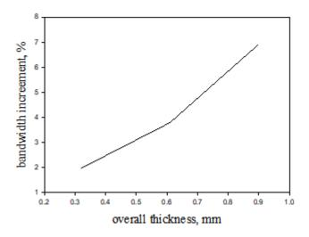
Figure 8. Relationship between bandwidth and total structure thickness.
