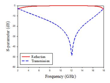
Figure 6. Transmission and reflection of FSS at 12 GHz.
