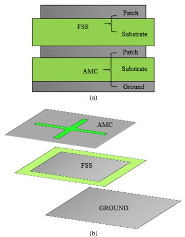
Figure 4. Dimension of AMC with the multilayer patch type FSS; (a) side view and (b) 3D view.
