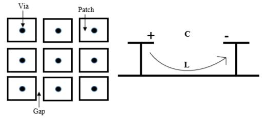
**Figure 1.** Basic AMC structure.
