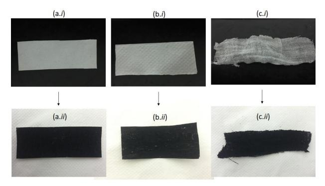
**Figure 1.** (a) filter paper, (b) tissue paper, (c) cotton cloth *pre*-cut to 6.5 cm x 2.7 cm dimension. (*i.* blank sheet, *ii.* After being deposited with PANI particles).
