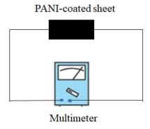
**Figure 2.** Schematic diagram showing the standard setup used to measure the resistance of the PANI-deposited sheet.
