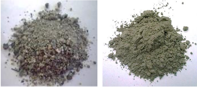
Fig. 1. Digital photo of (left) as-received palm ash (right) pulverized palm ash
