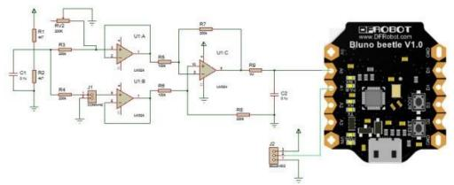
Figure 2. Schematic design of the hardware prototype.
