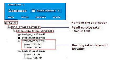
Figure 5. Firebase cloud database.
