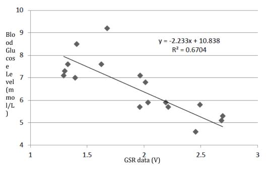
Figure 7. Correlation between blood glucose level and GSR readings.
