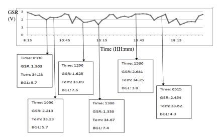
Figure 6. GSR graph with the respective blood glucose level for User 1.
