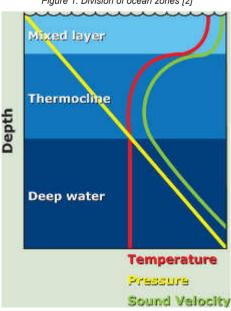
Figure 2: Temperature, pressure and sound speed variation with ocean depth [3]
