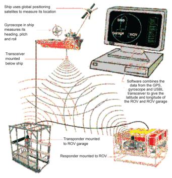
Figure 8: ROV positioning using USBL [8]
