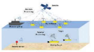
Figure 12: Proposed method of underwater acoustic postioning
