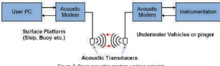
Figure 7: Basic acoustics modem working principle
