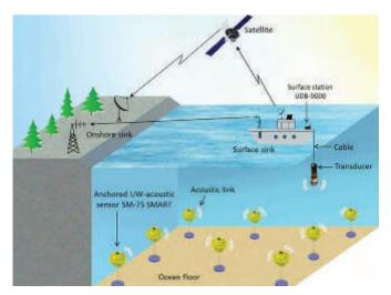
Figure 9: Underwater acoustic networking testbed [9]
