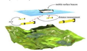
Figure 10: AUV cooperative localisation using mobile surface vehicle [10]
