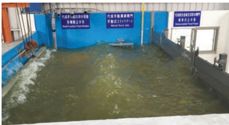
Wave testing in progress. On the right side is a demountable flood panel being the flood gate
