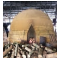
Kiln is sealed, leaving a small opening for burning fire wood
