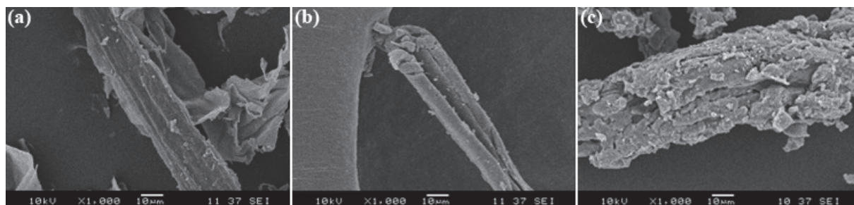
Figure 3. SEM micrographs of (a) untreated sample of coconut husk fibres, (b) pre-treated sample and (c) MCC sample at similar resolution.
