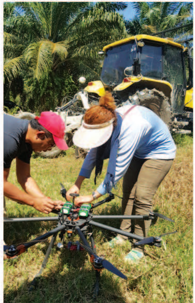
Figure 1: Turnigy 9XR octocopter UAV used for ganoderma detection, available at Department of Biological and Agricultural Engineering, Faculty of Engineering, Universiti Putra Malaysia
