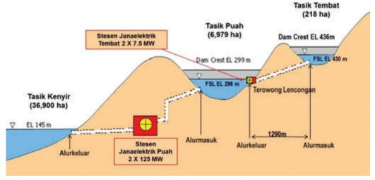
Figure 2: Cross-sectional view of the hydroelectric power scheme
