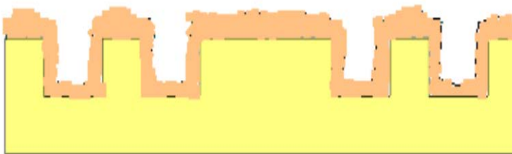
Figure 2. Alignment Mark Profile after Tungsten Deposition.
