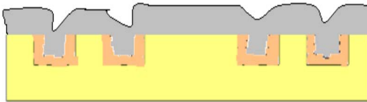
Figure 4. Post Aluminum/Metal Layer Deposition Profile
