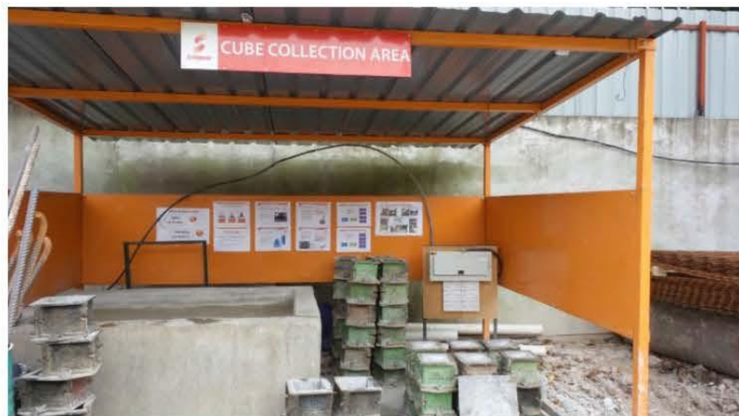
SunCon's standardised cube collection area at Sunway BRT Depot Project
