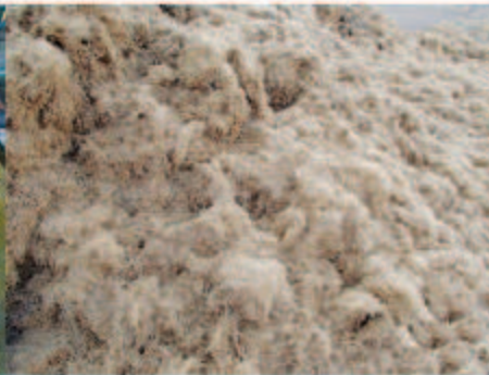
SHORT LOOSE FIBRE AS BOILER FUEL
